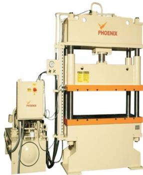
Other characteristics include a water to oil heat exchanger, track mounted adjustable limit switches and Allen Bradley electrical components. Pressure settings are selected electronically through a Micrologix 1000 programmable controller with 32 I/O. The operator interface is mounted on a movable T stand for flexibility.
