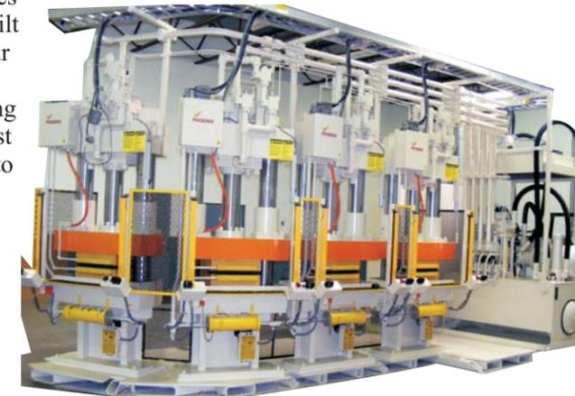
Each cell moves individually but is driven by one power unit. The press can be run in either manual or automatic mode. The cells are designed to build pressure on one press while allowing movement of the next press platen.
